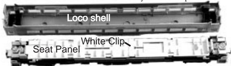
2. Gently remove the white clip that holds the seat panel in place. Remove the seat panel by pushing up gently from the bottom of the frame. The seat panel has clips underneath that are very easy to break so be very careful.
