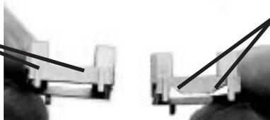
Modified lamp board clip with notches cut so that wires can pass through the clip.
