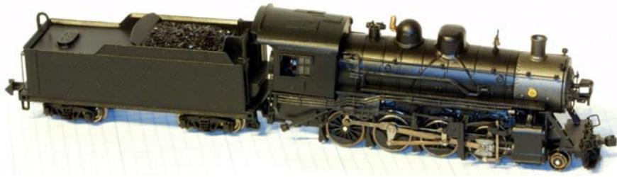
The decoder of choice for this locomotive is the Lenz LE10XF or the LE77XF. Digitrax DZ121 and DZ120 s are too long to fit inside the boiler shell without frame modification. It can be done but I do not recommend it.
