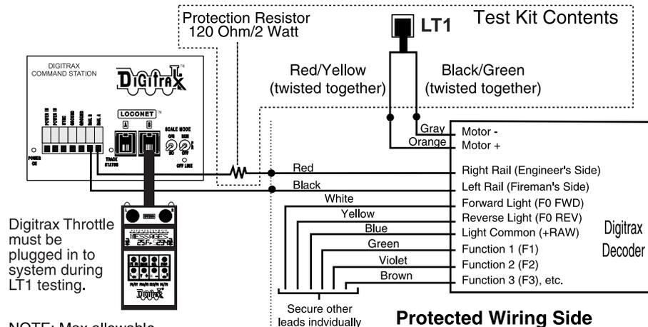
Digitrax Throttle must be plugged in to system during LT1 testing.
