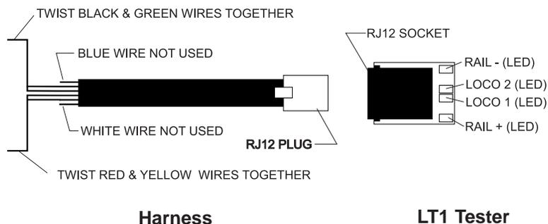
3. Hook up decoder as shown in *Diagram 2*.
